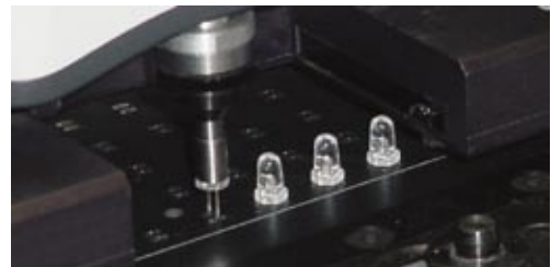
LED placement with customized nozzle.
