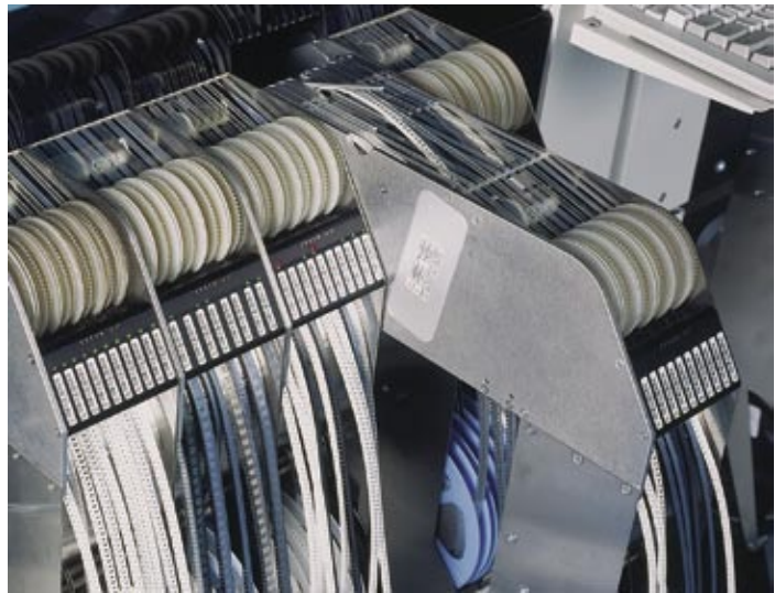
The cassettes are exchangeable while the machine is working. Refilling is possible directly on the machine.
