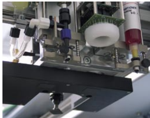
Optional single or double head dot dispensers increase the application range of the pick+place machine.
