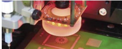
Top-down-Vision: Finds reference marks automatically.
