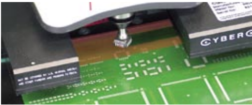
High speed: Fast on-the-fly Cyberoptics laser centring for chip and fine pitch placement.
