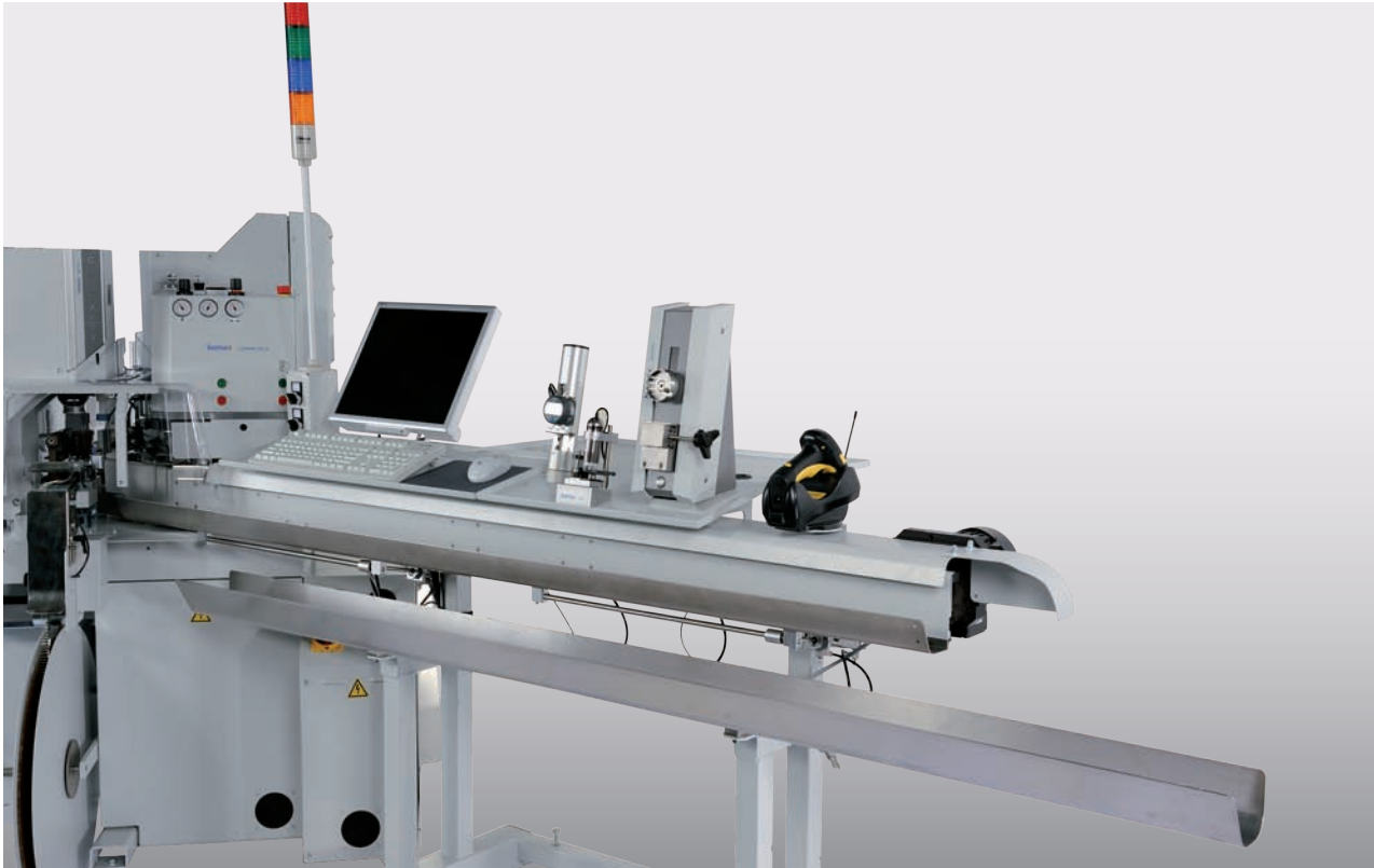
▲ Gamma 263 S with stainless steel tipping tray
