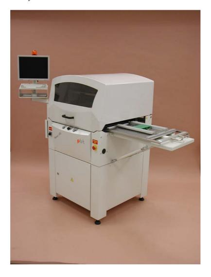
The interactive optical centring system consists from more precise X, Y, Theta adjusting mechanism controlled by 3 motors with linear position, two CCD cameras with the magnification 10x on quad of screen and sophisticated software which covers this system.
